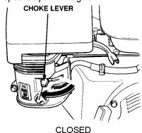
Figure 14. Choke Lever (Closed)
